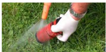
7. Tighten up disc filter by hand until securely tightened. Place back into filter body (will fit either way).
