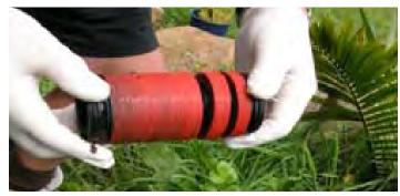
6. Wash out disc with garden hose or similar. Be sure to seperate discs and clean in between.
