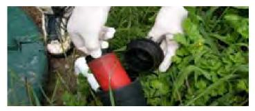
5. Loosen disc by unscrewing top off in an anti-clockwise direction.
